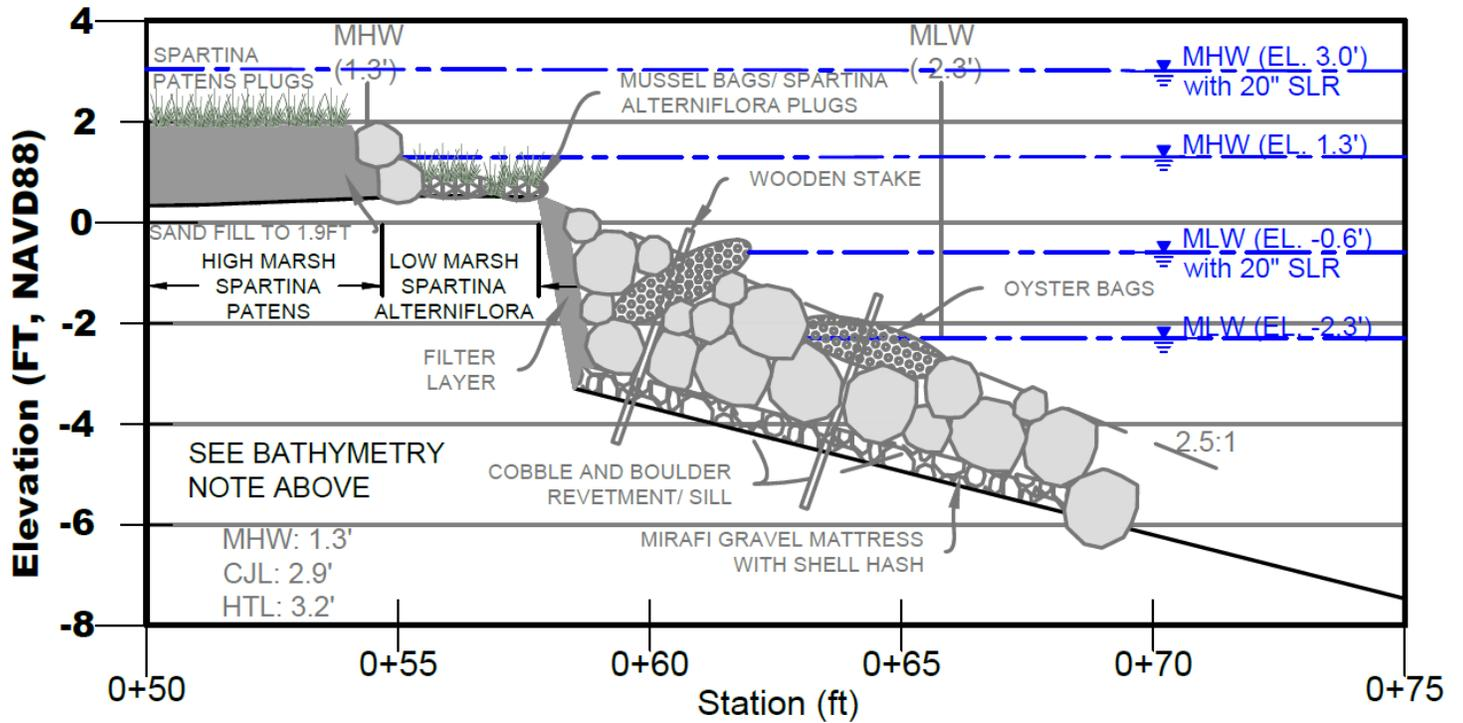
Note: The submerged bank slope and bathymetry is unconfirmed and highly dynamic. Supplemental bathymetric survey is required for final design.
