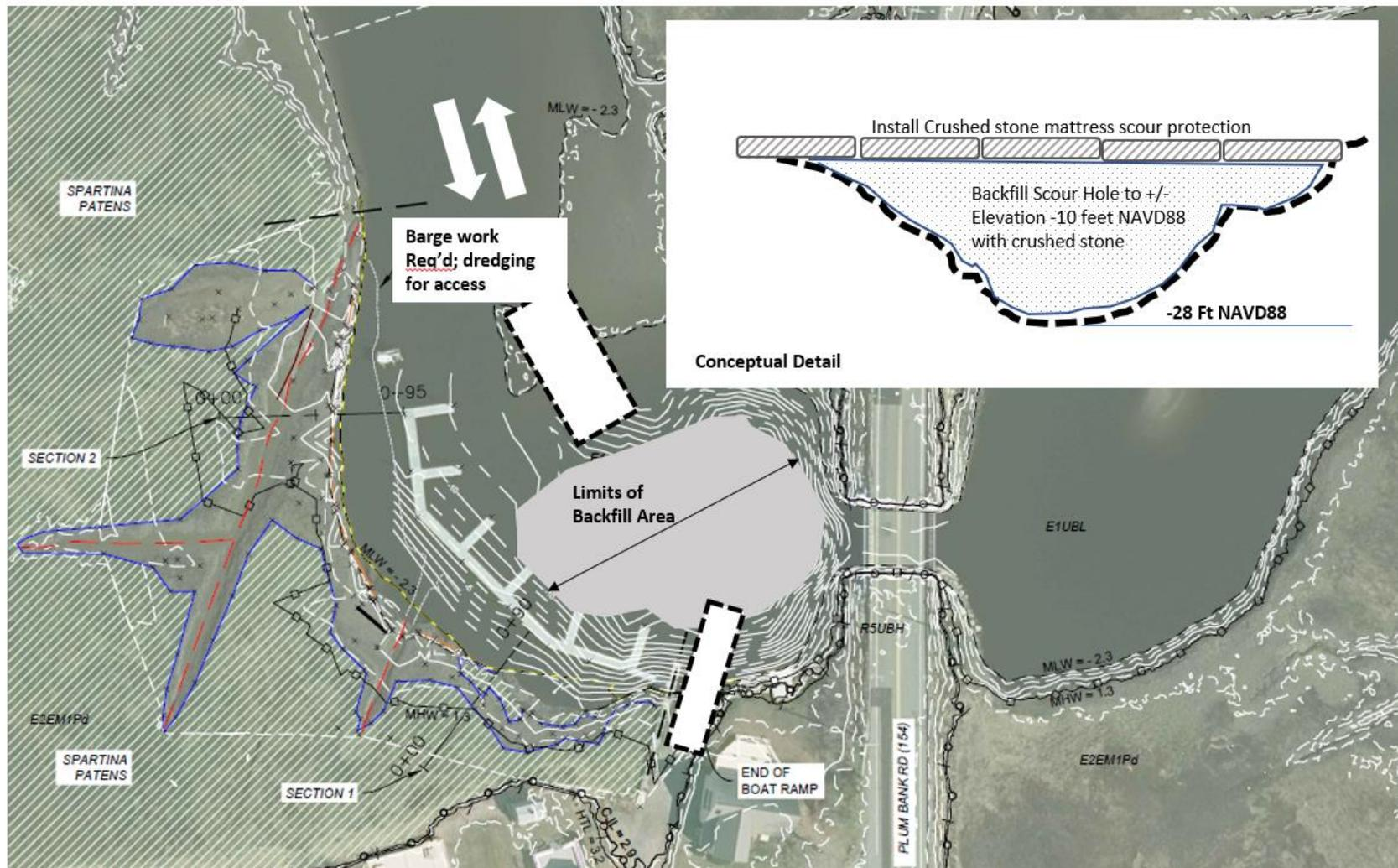
Figure 5: Supplemental Construction Conceptual Detail – Backfill and Scour Protection of Existing Scour Hole
