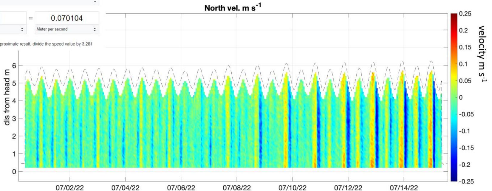
Distance from head of the instrument. The ADCP sits ~ 10 cm above the bed. Surface is marked in dashed black.
