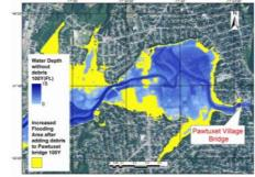
Figure 14: Effect of debris on the 100-yr flooding extent at the Pawtuxet Village brids
