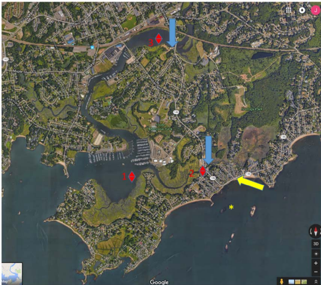
Figure 1. The coastline of Branford is shown using a GoogleEarth image with some locations of flooding on RT 146 indicated by the blue and yellow arrows. To understand how the water level in the Sound drives flooding we deployed instruments to measure sea level at the 3 locations shown by the red diamonds. We also deployed a wave sensor at approximately the location of the yellow *.
