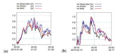
**Figure 11.** Comparison of significant wave height for two northerly storms at NH1 station outside the harbor. SWAN (blue), MIKE21SW (red), and observation (black) (a) 26 to 28 January. (b) 15 to 17 February.
