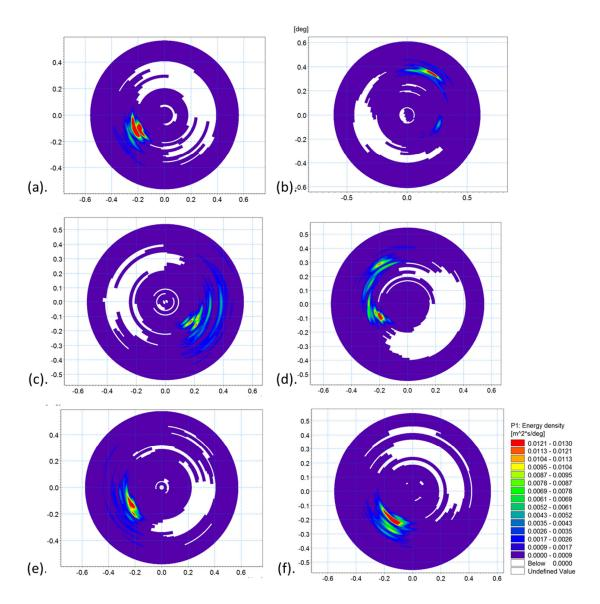
**Figure 4.** The two-dimensional wave spectra for important storms at NH1. As the majority of waves generates with local wind in central Long Island Sound, the spectrums are directionally wide. (a) 25 January; (b) 27 January; (c) 2 February; (d) 15 February; (e) 7 March; and (f) 2 April. The spectral wave models simulate wave diffraction for directionally wide spectrum better than directionally narrow spectrum, [2].
