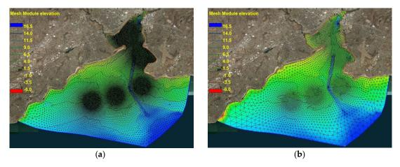
**Figure 3.** The optimum unstructured triangulate grids used for (a) SWAN with  $dx_{max} = 250$  m and  $dx_{min} = 25$  m and (b) MIKE21SW with  $dx_{max} = 500$  m and  $dx_{min} = 50$  m; SWAN required a finer grid to reach the optimum condition. The spatial smoothing of the grids is the same. The grids were refined around the breakwaters, three densification zones, and in the harbor.
