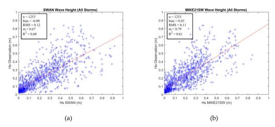
**Figure 10.** Comparison of scatter plot and statically parameter between observed and simulated significant wave heights from SWAN (a) and MIKE21SW (b) for all storms. There was no substantial difference between the performance of the models. *Bias* was better for SWAN and *RMS*, the slope best fitted line and  $R^2$  were better for MIKE21SW.
