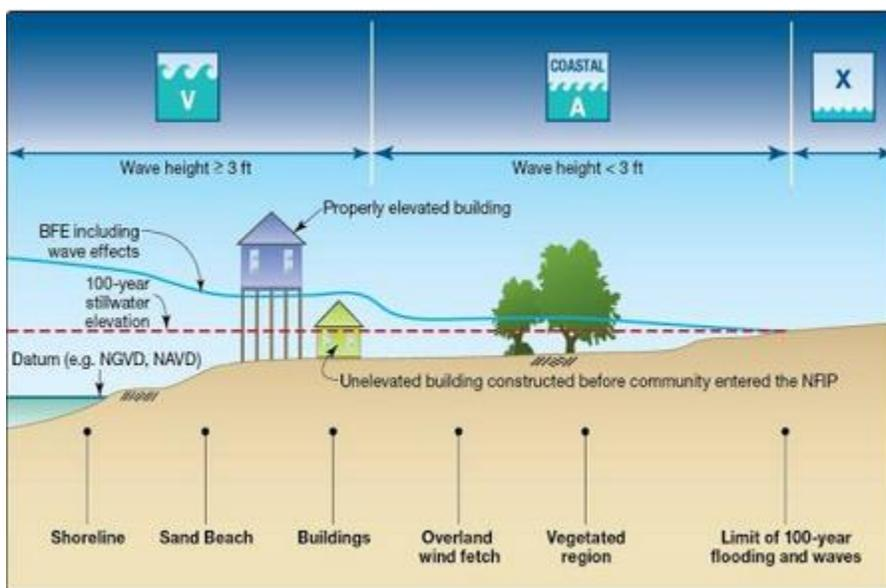
*Schematic of FEMA flood zone designations for coastal V, A and X zones (source: [FEMA Region II Coastal Analysis and Mapping, Coastal Mapping Basics](#))*
