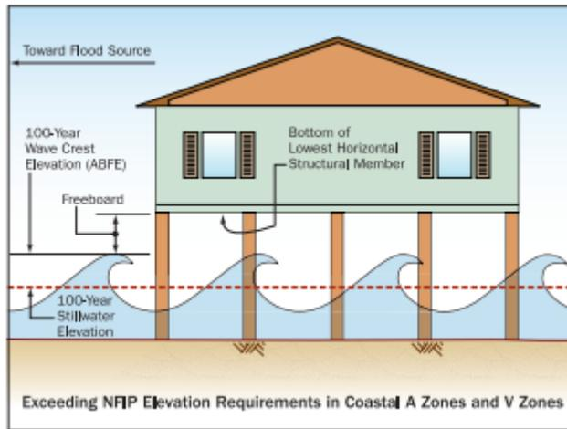
If you are located in a flood zone, your town may require that the lowest structural part of your house be a minimum of one foot above the Base Flood Elevation (BFE). This is typically the minimum standard, but check with your local zoning enforcement officer for local ordinances. (Source: FEMA [Designing for Flood Levels Above the BFE, Home Builders Guide to Coastal Construction, Technical Fact Sheet 1.6](#))
